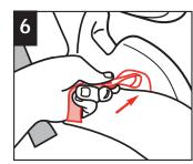
Push LATCH hook through the other rearfacing belt path slot.
